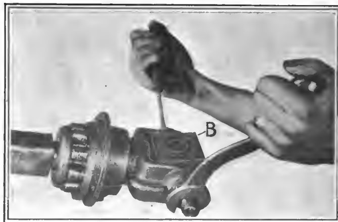
Fig. 2—Manner of adjusting for play in universal joint with a wrench and screw-driver
